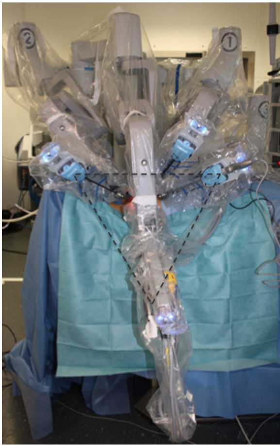
Fig. 3. Operating position of the robot (right-sided procedure). Triangulation of the main instruments: camera, Maryland (arm 2) and Ultracision (arm 3). The Prograsp forceps (arm 1) is positioned between the endoscope and the instrument at the caudal extremity of the incision.
